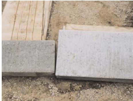
Color comparison of a block made without (left) and with (right) slag cement.
